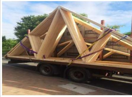
3. Pasquill will supply truss packs secured to the trailer with blue 3 core rope. You shall familiarise yourself with which rope attaches which pack to the centre bars.
